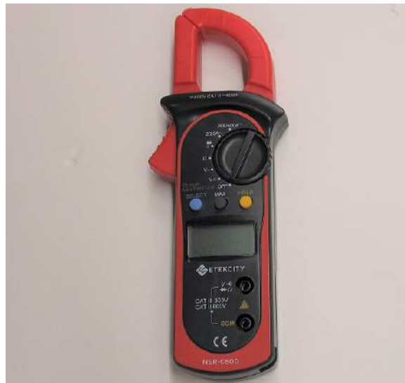
A standard clamp meter with spring-loaded jaws for measuring large AC currents.
