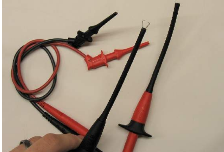
Mini grabbers, one integrated into the leads and the other is an attachment for the end of an extension cable.
