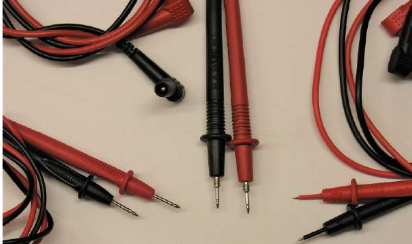
A close-up of several 'standard' meter leads. They include the default standard, the one with a small threaded section, and the insulated fine-point tips from left to right.
