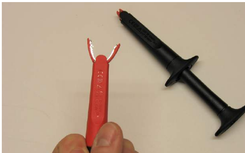
The syringe-style action of a jaw adapter for the end of an extension cable.
