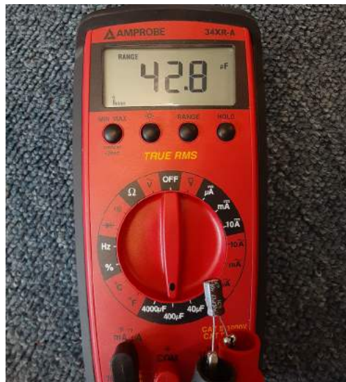
Measuring capacitance. Note the connection of the meter leads and the symbol indicated, matching the negative (-) symbol on the capacitor.
