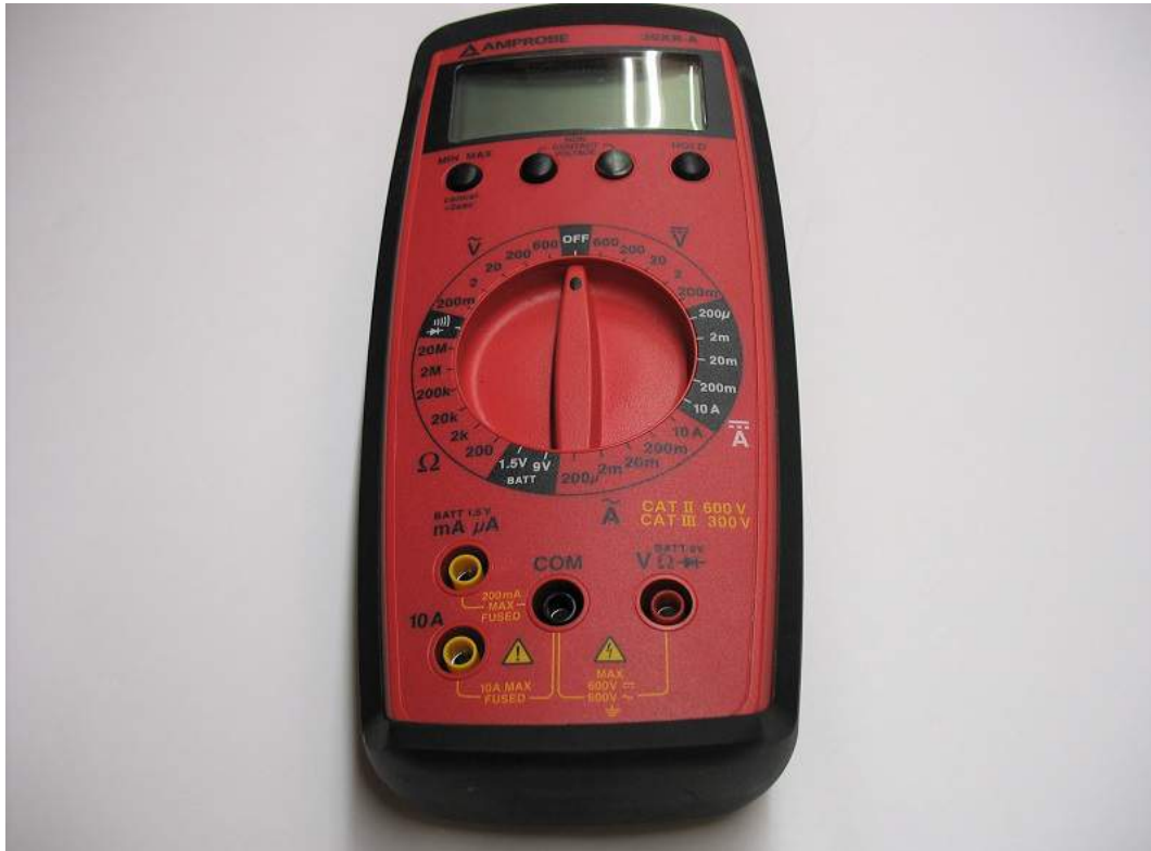
A digital multimeter, although this one does not automatically range through relative scales of each function, in other words, it's non-autoranging.
