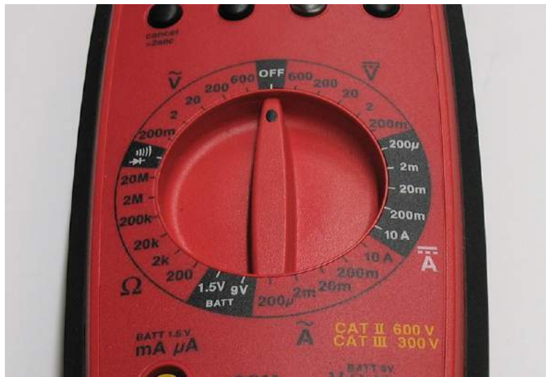
A manual ranging meter showing selections of 200 mV through 600 V as well as ranges for current and resistance.
