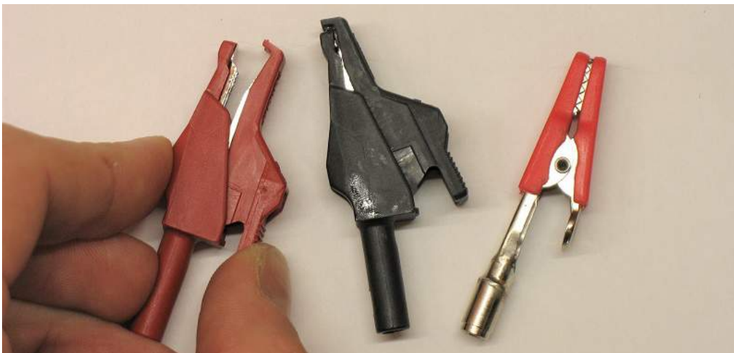
A few alligator clip ends. Note that the exposed metal one usually has an insulated jacket over the top, but it's been removed to show what it looks like inside.
