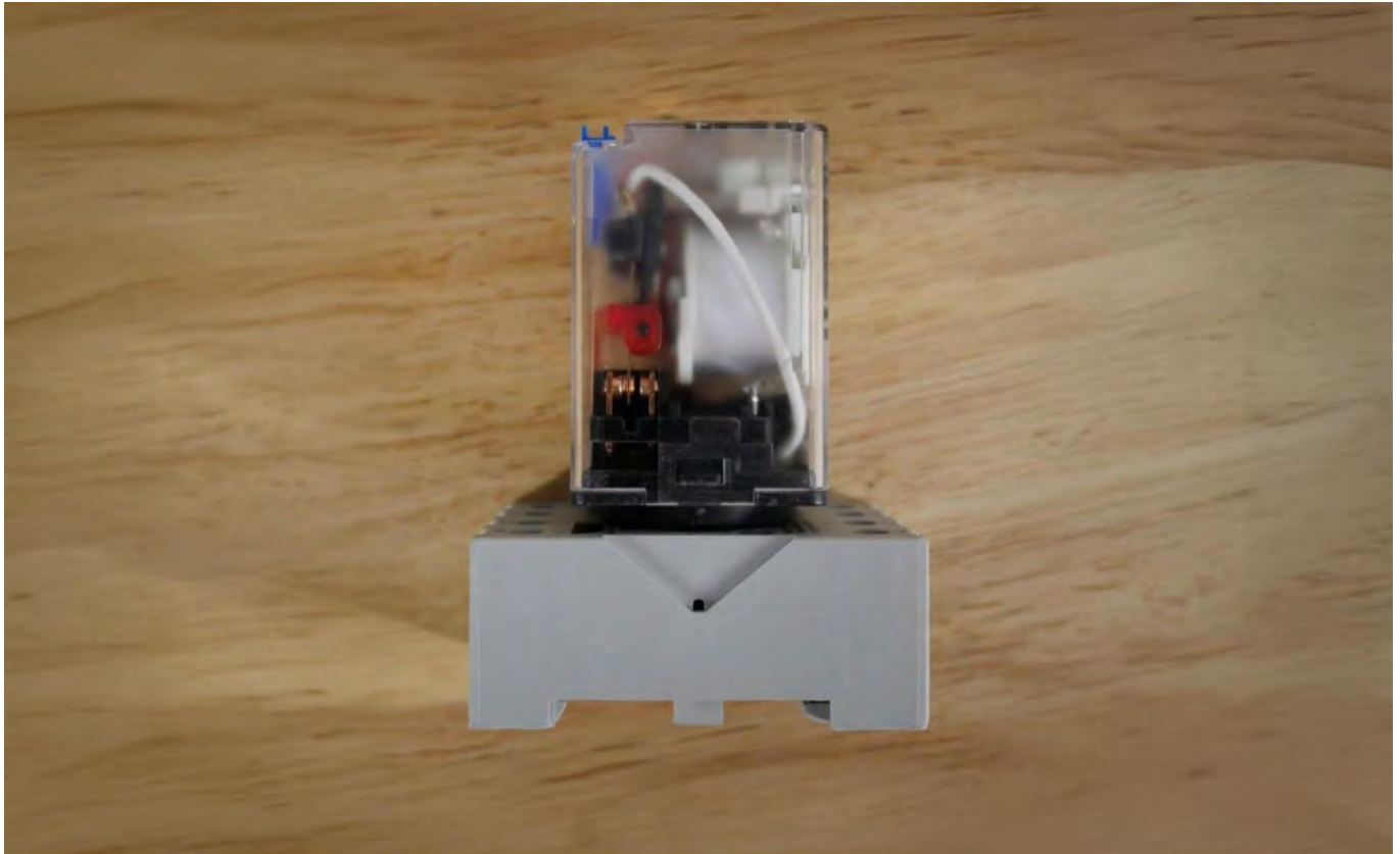
A DPDT relay, which includes a blue test switch at the top, allowing manual toggling between the NO and NC contacts, which can be seen through the transparent side casing.
