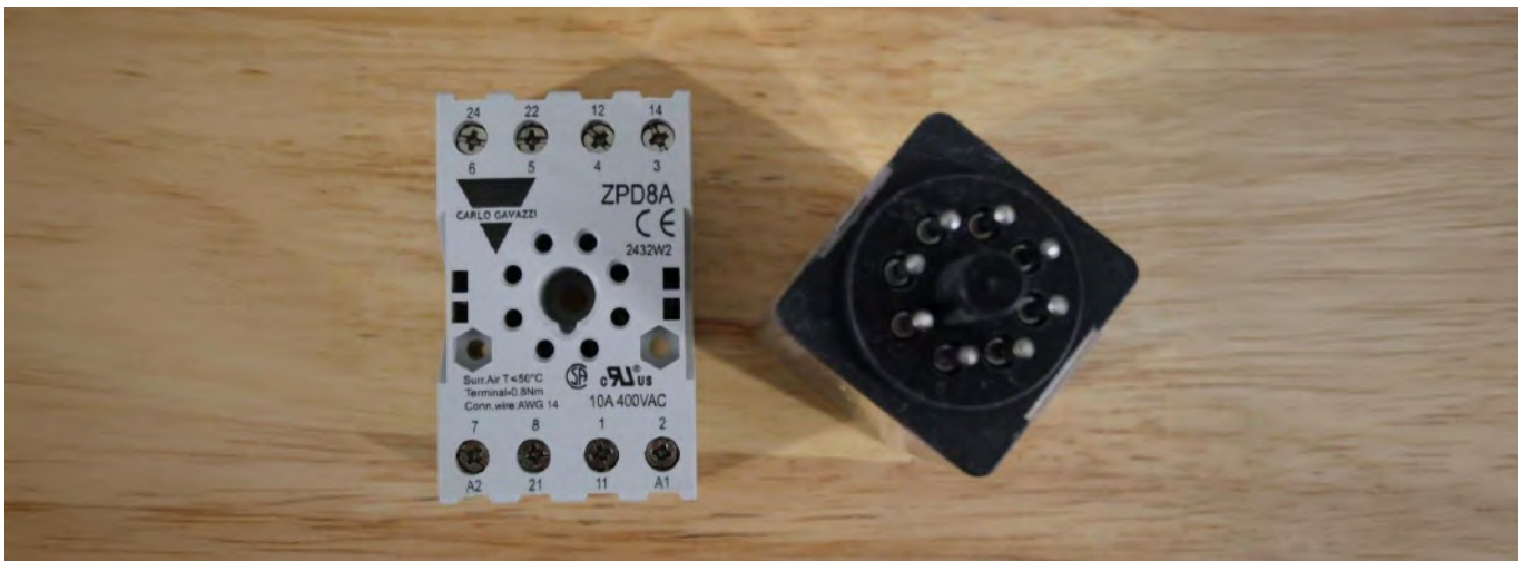
A DPDT octal relay with socket numbers showing both NEMA and IEC standards.
