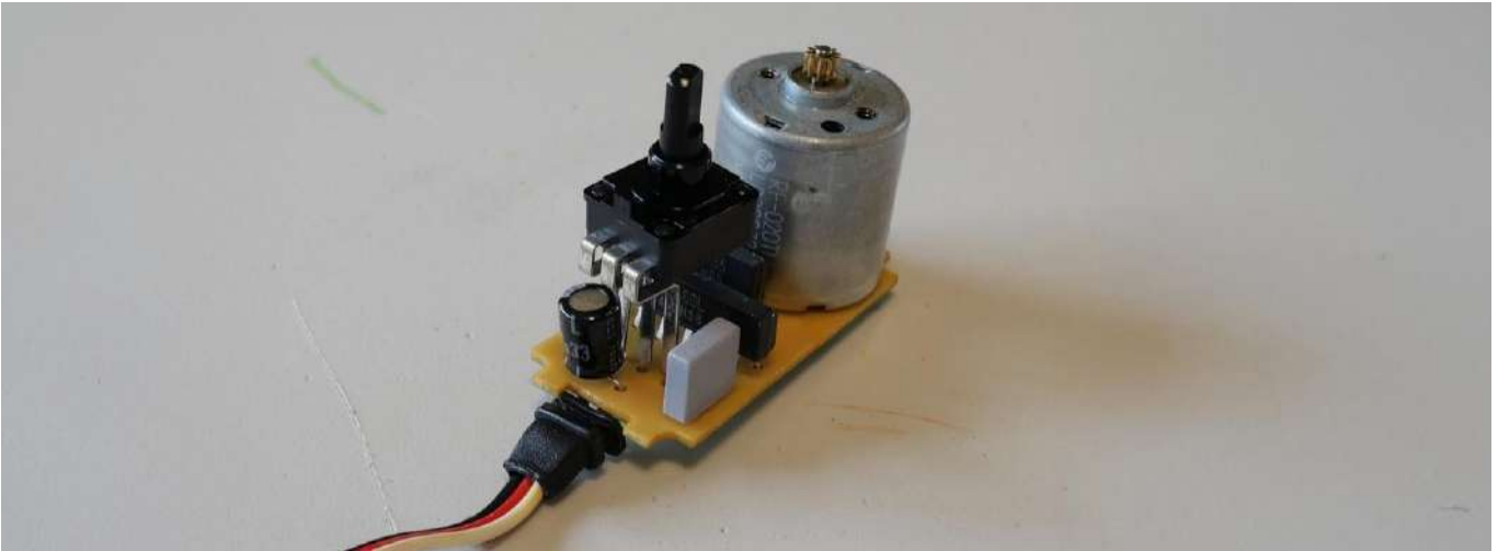
A potentiometer is linked to the DC motor in many small servo mechanisms.
